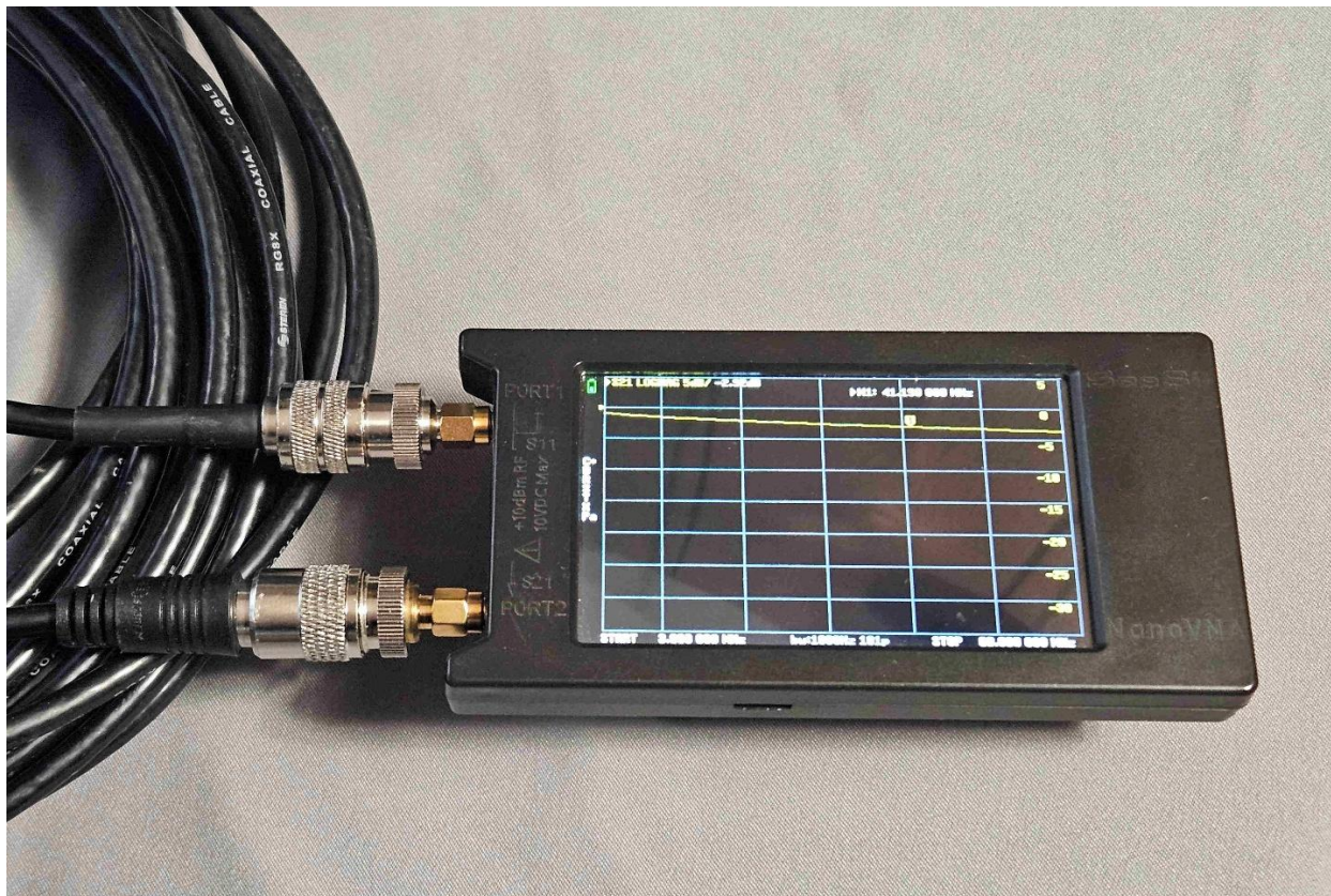
FIG 5: Measurement of losses for 50' coax cable and two PL-259 connectors.
